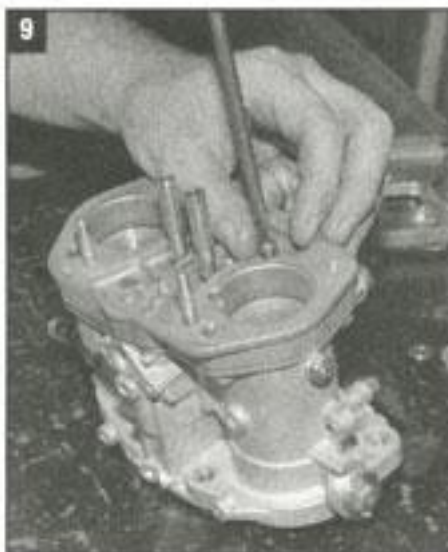
11. The horizontal discharge tubes provide increased air flow and improved air/fuel emulsification when used on port ram intake systems. The taller, top inlet idle air jets help eliminate plugged idle jets because most of the dirt and road grime that finds its way into the system is pulled into the idle jets from the top surface of the carburetor.
