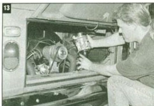
13. Scott installs the updated 40DRLA carburetors on "Ole Blue." C.B.'s VW Van sees the dual purpose of rolling test bed and delivery truck, the air filters and crankcase vent tube will be fitted after the carburetors and linkage are put into sync.
