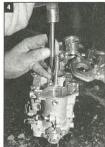
4. Your up-to-date kit includes four lead plugs. They look like fishing sinkers but are actually used to plug those troublesome idle air holes on top of the carburetor. Use a blunt punch and ballpeen hammer to plug the brass air inlet holes.
